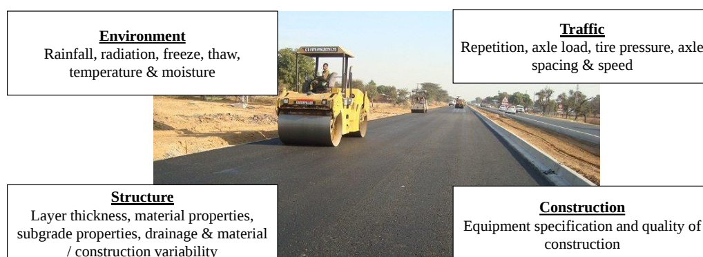
Figure 2: Factors Affecting Flexible Pavement Performance
