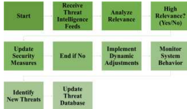
Figure 2: Continuous Threat Intelligence Feeds Integration (CTIFI) algorithm
