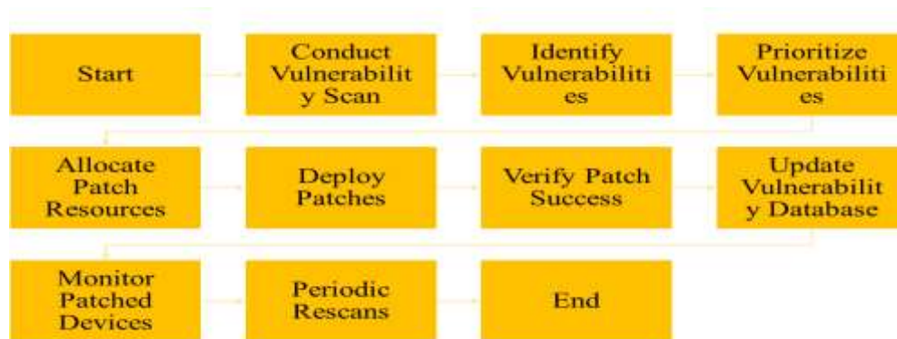
Figure 4: Vulnerability Scanning and Patch Management (VSPM) algorithm
