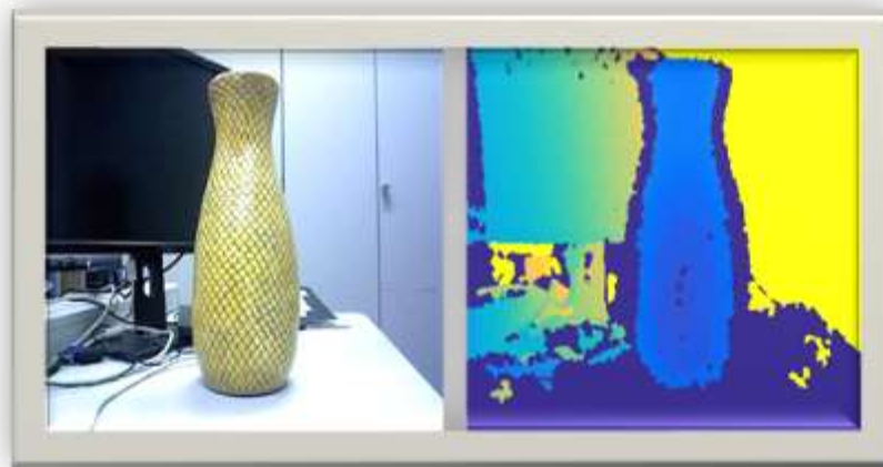
Figure 3: The input RGB and depth image of a vase. The depth map is visualized using colors from blue (near) to yellow (far), where the missing areas and quantization effects can be noticed.
