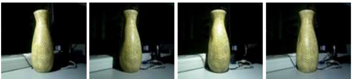
Figure 5: Illustrations for the obtained color images of a vase from various light directions with a white LED light. Even the phone flashlight is sufficient for giving various lighting.
