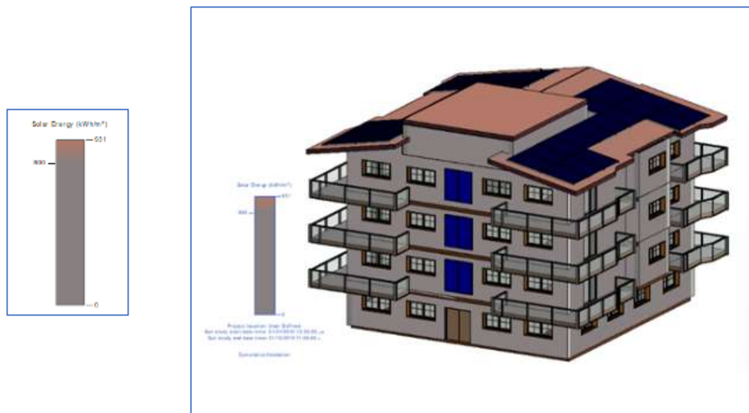
Figure 10: Sun Analysis Results and PV Energy Production for the Second Situation (Changing building material)
