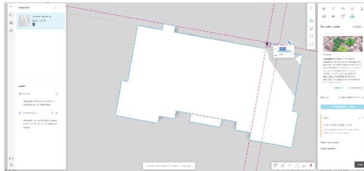
Figure 1: Shows the creation of the three-dimensional model of the building within Autodesk Forma - The number of floors, their height, and the building area are specified, along with the building's function.
