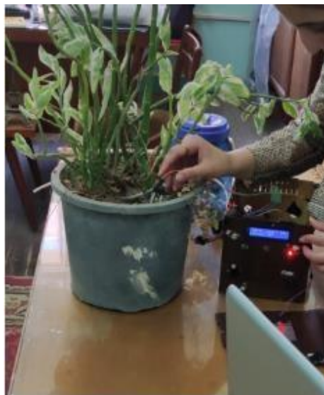
Figure 10. Determination of soil moisture using monitoring system
