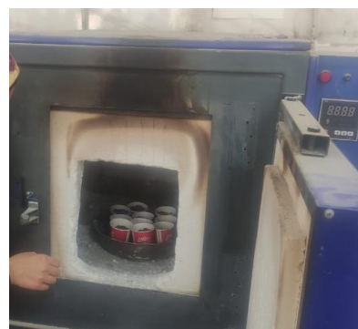
(b) Drying the soil samples
