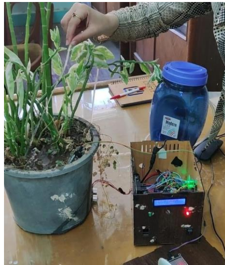
Figure 13. Pumping water into the soil when the moisture content is low
