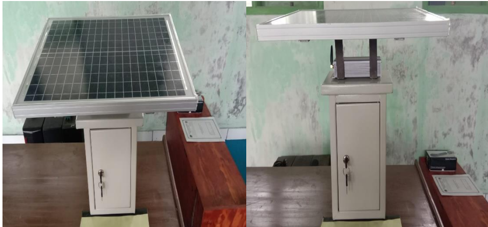
Figure 3. Product PM monitoring system-using IoT based on the Solar panels
