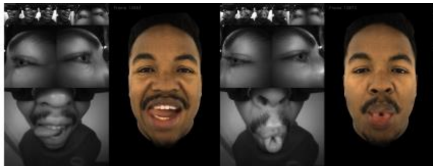
Figure 9: Example results of [34]. For both examples, the images on the left in gray are the input, and the images on the right are the rendered mesh. The larger grayscale images are the non-augmented input images from the actual headset, and all of the smaller grayscale images are the additional views.
