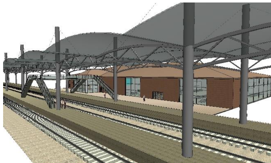
Fig.3 Assembling Revit models of passenger platform, passageway, canopy, and passenger building
