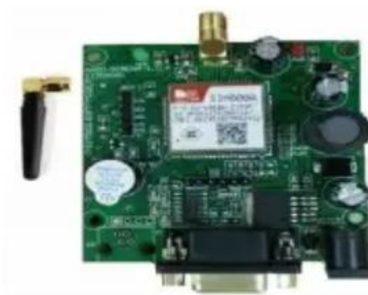
Figure 4: GSM 900 module of our system
