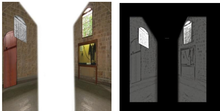
Figure 22: the effect of natural lighting (sunlight) from the southern elevation on the critical wall, which is the interior wall of the exhibition halls facing the windows in Lattakia Museum.
