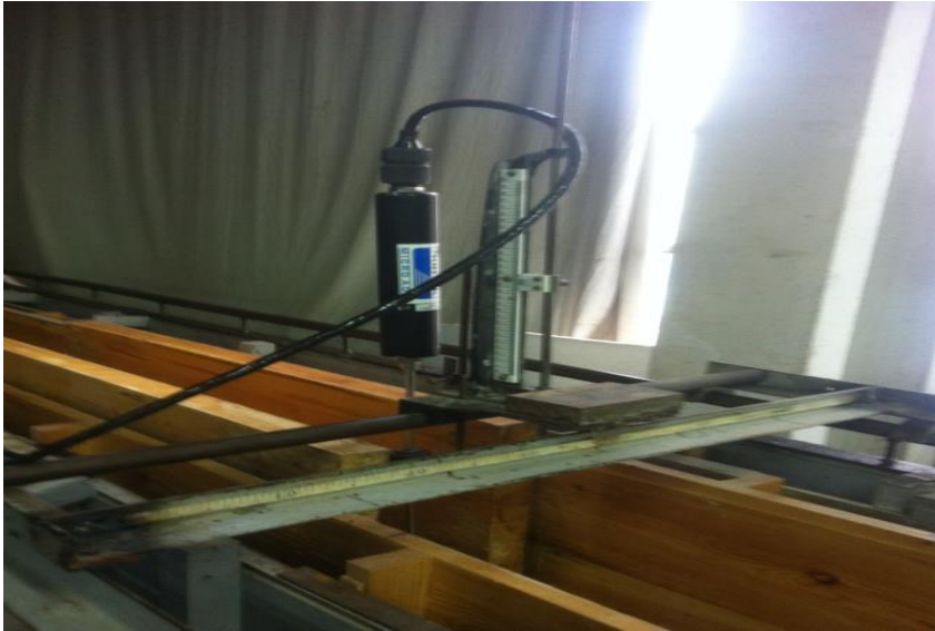
Figure 3: Acoustic Doppler Velocimeter.
